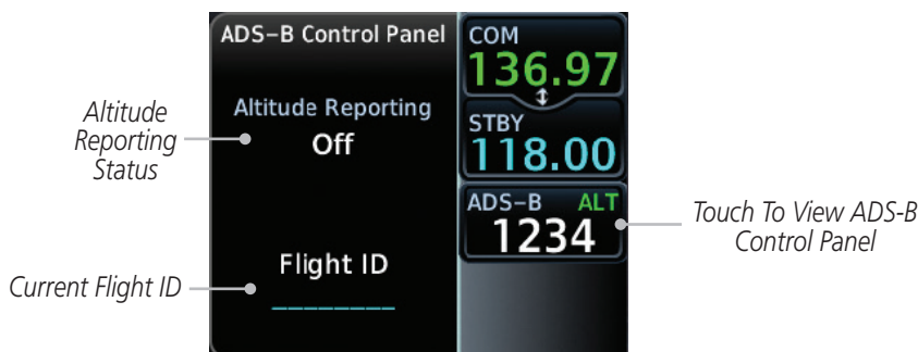
Figure 2-13 ADS-B Control Panel
