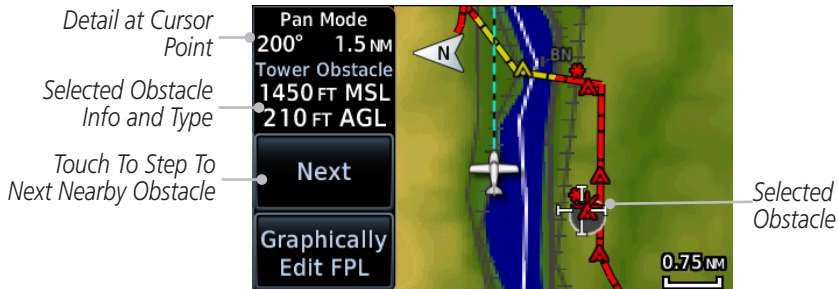
Figure 8-24 Point Obstacle Detail
