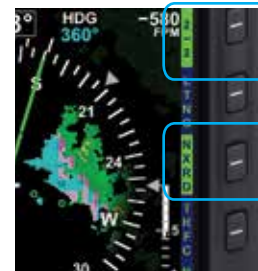
Figure 4-123 Data Link Weather Enabled
