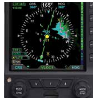
Figure 4-114 Navigation Display Showing Hazard Awareness
